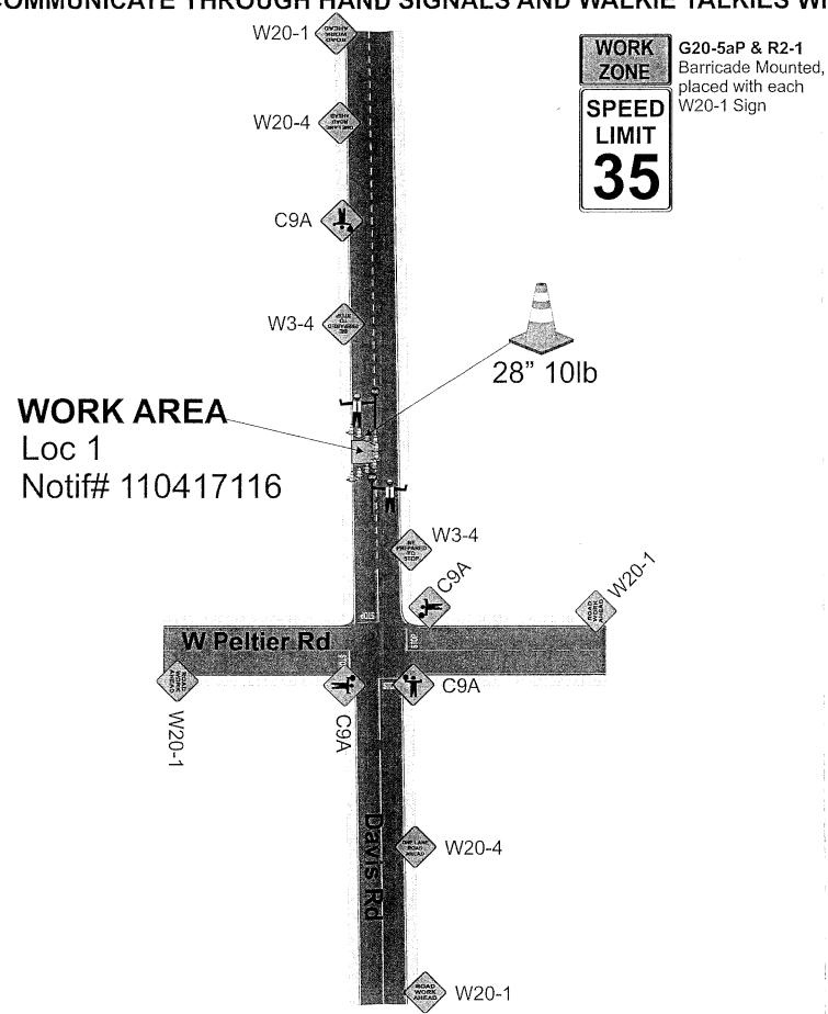
SIGN SPACING TAPER TANGENT SPEED TAPER 125 30 180' 30 60 35 35 70 245 500' 40 320' 40 45 540 600' SHOULDER(1/3taper) BUFFER(1/2taper)
